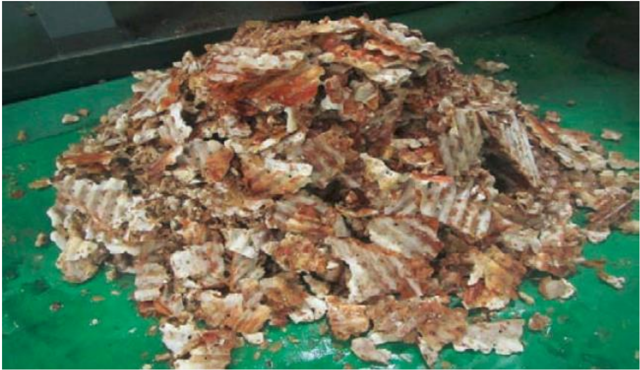
Removed soft scale without use of chemicals
