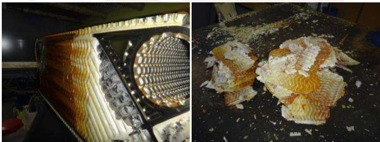
Figure 2. The Fresh Water Generator plate and the removed limescale
